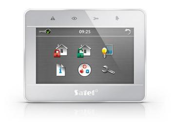
**INT-TSG** also provides an easy access to the information on current system status. Thanks to the status screen customization possibilities, a single glance at the display could be enough to find out if the system is armed, if the outdoor lighting is on or if the garden watering is currently on. The status screen may also be used for the picture gallery.
